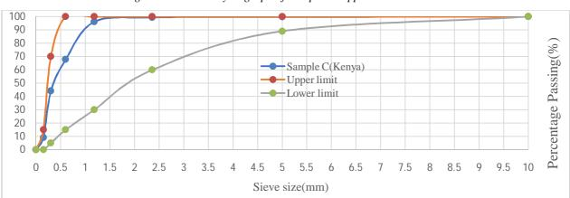
Figure 4: Sieve analysis graph of Sample C-Upper Limit-Lower limit
